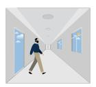
With sufficient daylight, the sensor keeps light OFF even when motion is detected
