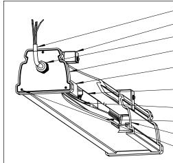
72" BLACK, 18AWG, 600V, 5-CONDUCTORS POWER CORD 316 STAINLESS STEEL SURFACE MOUNT BRACKET
