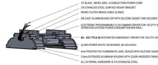
72" BLACK, 18AWG, 600V, 5-CONDUCTORS POWER CORD 316 STAINLESS STEEL SURFACE MOUNT BRACKET NICKEL PLATED BRASS CABLE GLANDS
