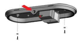
5. Reconnect the battery paying attention to the polarity as shown. Secure reflector in place. Aim the lamps to desired position and snap the lens in place.
