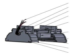
72" BLACK, 18AWG, 600V, 5-CONDUCTORS POWER CORD 316 STAINLESS STEEL SURFACE MOUNT BRACKET NICKEL PLATED BRASS CABLE GLANDS
