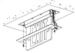
**Pendant Mount:** The pendant kit consists of a single pendant stem in standard 12", 24" and 48" lengths (1/2" IP) and a flat ceiling canopy. White and black finishes are standard. Consult factory for custom lengths.
