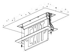
**Pendant Mount:** The pendant kit consists of a single pendant stem in standard 12", 24" and 48" lengths (1/2" IP) and a flat ceiling canopy. White and black finishes are standard. Consult factory for custom lengths.
