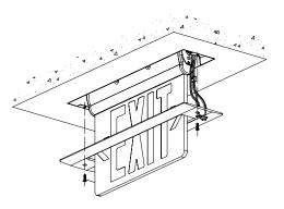
The recess kit allows for the standard surface mount **CRV2** to be easily recessed into a ceiling or a wall. The standard unit snaps into the recessed backbox and is securely held in place while wiring is completed.
