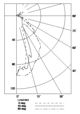
Meets NFPA 101 Requirements for: 12' center-to-center spacing - 3' path of egress 1' from wall - 7 1/2' mounting height.
