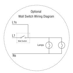
Wall Switch Option (WS): Provides an internal relay which allows two circuits of emergency power to the lights regardless of the wall switch position (on or off).
