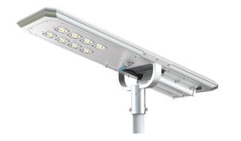
APPLICATION: The BLS-6A is ideal for temporary lighting, pathways, parking areas, public walkways, parks and roads. The LUCE SOLARE BLS-6A is a solar street and area lighting solution that integrates the solar panel, battery and LED module into a single low-profile fixture. BLS-6A utilitizes battery technology that will not drain below 10% capacity to ensure reliable re-charge for maximum performance.
