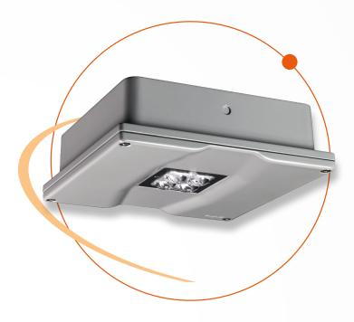
The Pluraluce® SQUARE RECESSED Unit is rated for indoor installations and is configured with a two wire 120-347VAC 50/60Hz input. The steel trim comes standard in a white powder coat with optional painted or brushed finishes. Offered in HT, SE and SA configurations; the Pluraluce® SQUARE RECESSED Unit provides up to 845 lumens. Designed for recessed mounting in non-IC installations only.
