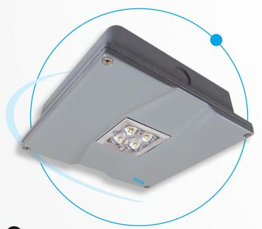
The **Pluraluce**® **INDOOR Unit** is rated for indoor installations and is configured with a two-wire 120-347V 50/60Hz input. The aluminum cover comes standard in a white powder coat with optional painted or brushed finishes. Offered in HT, SE and SA configurations; the **Pluraluce**® **INDOOR Unit** provides up to 845 lumens. Flexible mounting options include: surface wall, ceiling and pendant.
