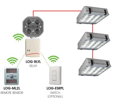
**APPLICATION:** LOG-RLYL is ideal for single or multiple fixtures on/off or dimming control applications. LOG-RLYL is ideal to use in most damp/wet locations based on product rating.
