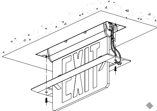
The recess kit allows for the standard surface mount **CURVA** to be easily recessed into a ceiling or a wall. The standard unit snaps into the recessed back box and is securely held in place while wiring is completed.
