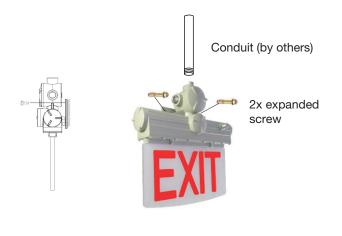
4. Install the two expanded screws to the holes (shown above). Attach pole for pendant mount (optional).
