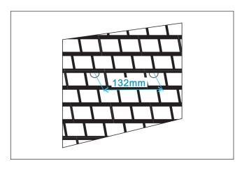
Drill two 8mm holes for expanded screws 132mm apart.
