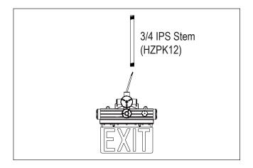
1. Thread the AC cable through the pendant pole.
