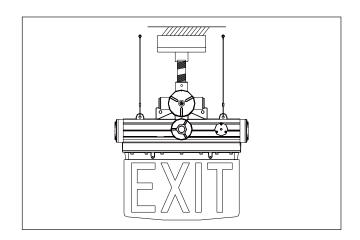
Install the fixture to junction box. Connect the AC cable; black cable to L, white cable to N, green cable to grounding.
