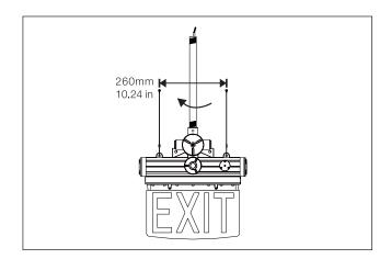
3. Drill two Ø10mm holes for the metal wires into chosen surface and tighten the skid-proof screw.
