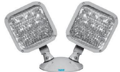
The **BRH** remote is available for indoor or outdoor applications. **BRH** remote is designed with high-performance chrome-plated metalized reflector and provides optimal light distribution. Fully adjustable LED heads ensure emergency lighting performance, accurate positioning and reduced maintenance. **BRH** is multivoltage (3.6V, 6V, 9.6V & 12V). Each head totals 1W. High output remote heads optional (1.5W). The operating temperature is from -22°F up to 104°F (-30°C up to 40°C).
