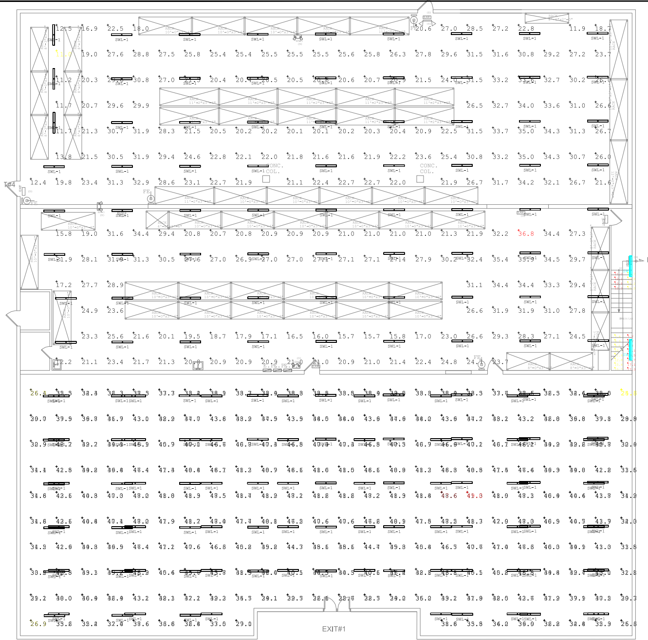
01 STORAGE SOLUTION- LUMINAIRE LOCATION & CALCULATION POINTS NTS
