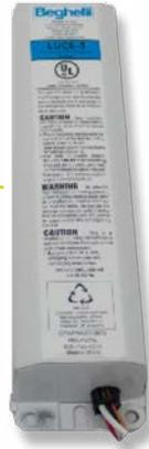
■ **Installation:** The **LUCE-5** emergency ballast does not affect normal fixture operation and may be used with either a switched or unswitched fixture. If a switched fixture is used, an unswitched hot lead must be connected to the emergency ballast.
