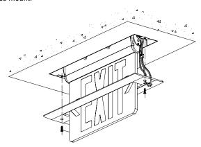
The recess kit allows for the standard surface mount **CURVA** to be easily recessed into a ceiling or a wall. The standard unit snaps into the recessed back box and is securely held in place while wiring is completed.
