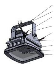
3mm THICK STEEL MOUNTING BRACKET (ADJUSTABLE) WITH GRAY POWDER COAT FINISH IS STANDARD.
