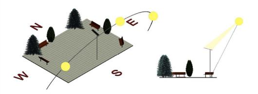
These graphics illustrate Luce Solare orientation, in which the fixture can absorb the maximum solar energy from the sun (south 100% - refers to product specs).
