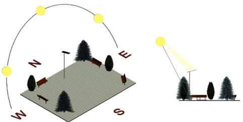
These graphics illustrate Luce Solare orientation, in which the fixture can absorb the maximum solar energy from the sun (north 100%).
