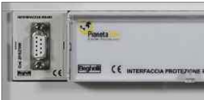
Local supervision system with RS485 wired connection
