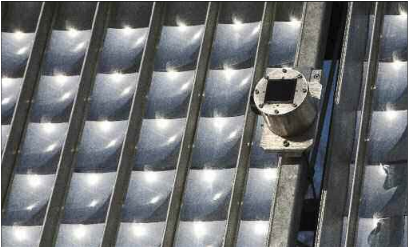
Tracking system with solar camera
